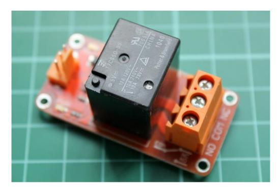
A **relay** is an **electrically operated switch** that allows you to turn on or off a circuit using voltage and/or current much higher than the Arduino could handle. There is no connection between the low voltage circuit operated by Arduino and the high power circuit. The relay protects each circuit from each other.
