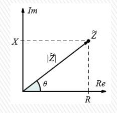
» When a circuit is driven by DC there is no distinction between impedance and resistance (impedance with phase angle to be zero.
