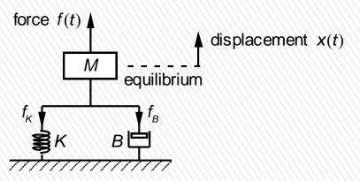
Net force on mass upwards =  $F(s) - (F_{\kappa}(s) + F_{B}(s))$ Apply Newton 2<sup>nd</sup> Law:  $F(s) - KX(s) - BsX(s) = Ms^{2}X(s)$
