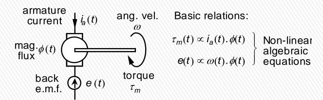
Therefore:  $\tau_m(s) = kI_a(s)\varphi(s)$  and  $E(s) = k\omega(s)\varphi(s)$
