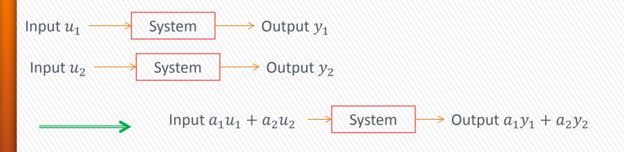
Superposition Principle and Linear Systems
