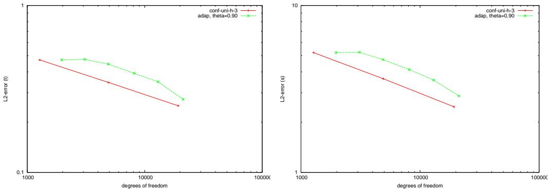
Figure 6.123: Stokes (2d-FEM-BEM):  $\|t - t_n\|_{L^2(\Omega)}$  (left) and  $\|\sigma - \sigma_n\|_{L^2(\Omega)}$  (right).
