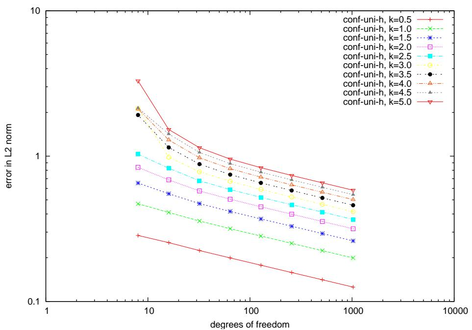
Figure 2.14: Helmholtz: Weakly singular integral equation, convergence in  $L_2$ -norm
