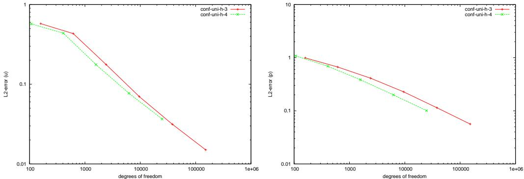
Figure 5.89: Stokes (2d-FEM, mixed b.c.):  $\|u - u_n\|_{L^2(\Omega)}$  (left) and  $\|p - p_n\|_{L^2(\Omega)}$  (right).
