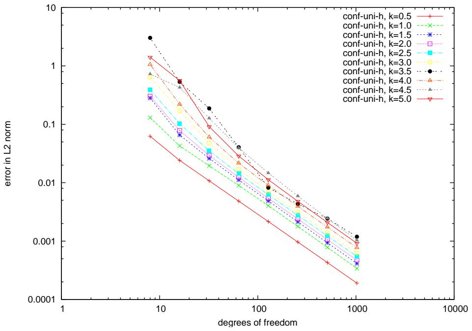
Figure 2.15: Helmholtz: Hypersingular integral equation, convergence in  $L_2$ -norm
