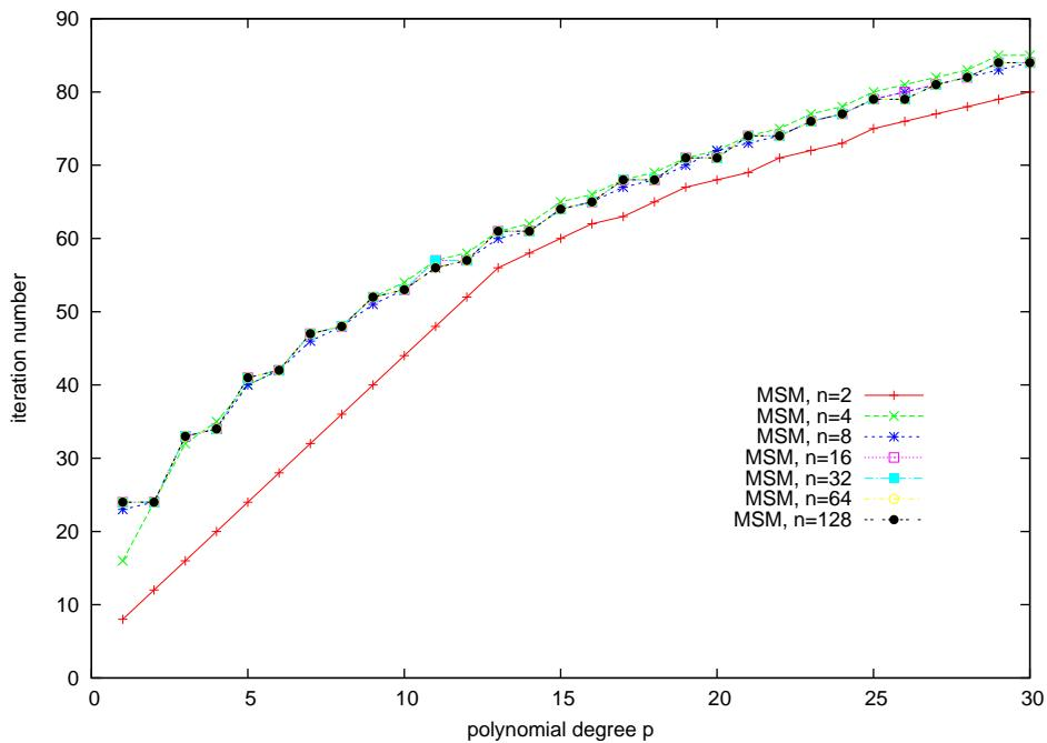
Figure 2.27: Weakly singular integral equation, p-version, iteration numbers
