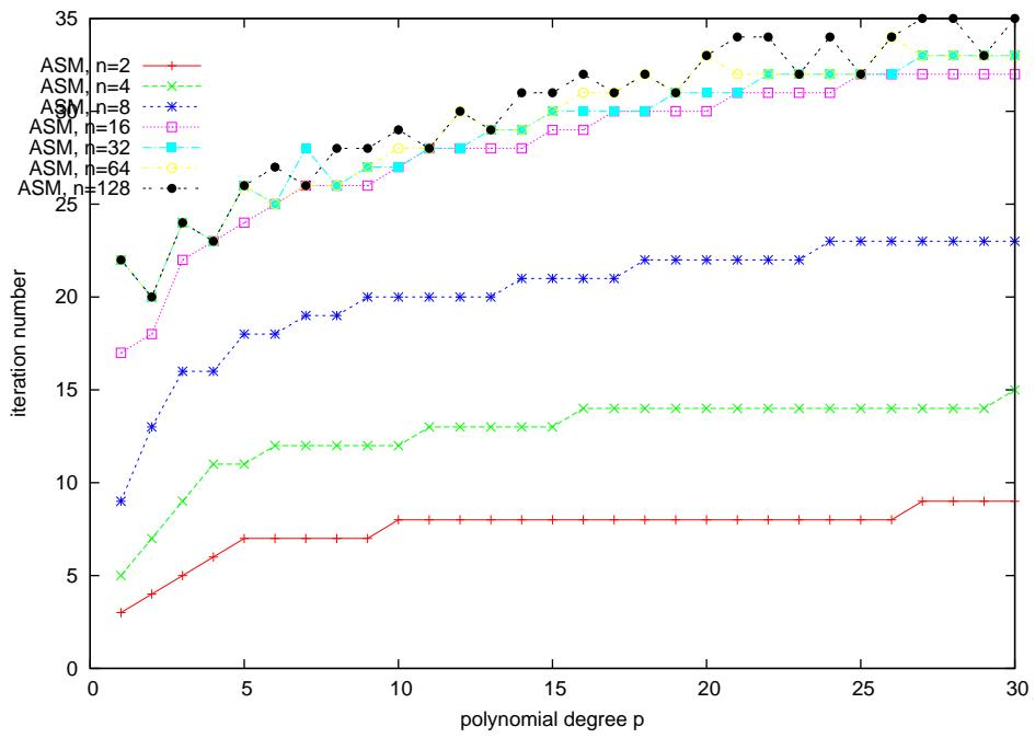
Figure 2.33: Weakly singular integral equation, p-version, iteration numbers
