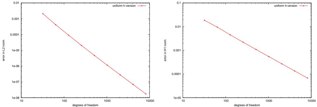
Figure 2.10: Lame(Neumann, interior, displacement): Steklov-Operator, convergence in  $L_2$ -norm and  $H^1$ -norm
