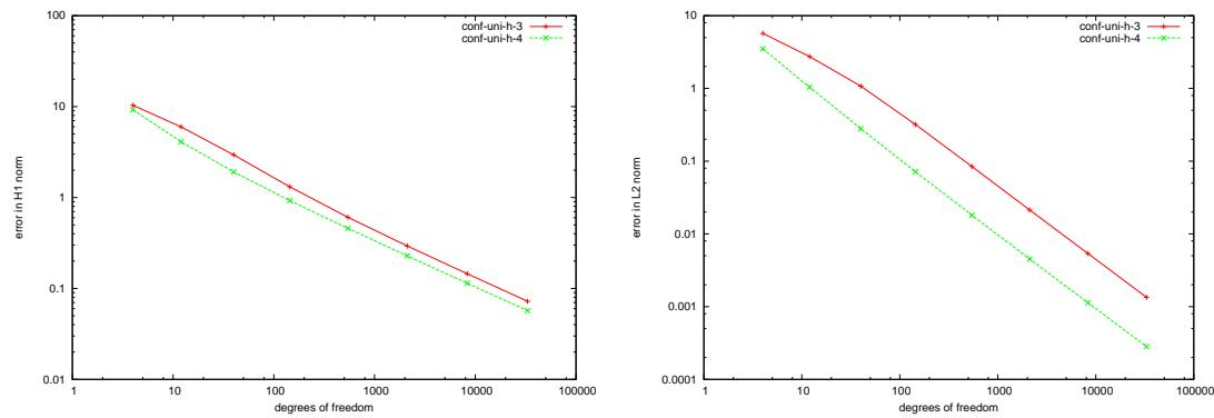
Figure 5.72: Error in  $H^1(\Omega)$ -norm (left) and in  $L^2(\Omega)$ -norm (right)
