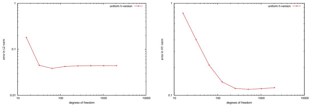
Figure 2.22: Stokes(Neumann): First kind integral equation, convergence in  $L_2$ -norm and  $H^1$ -norm
