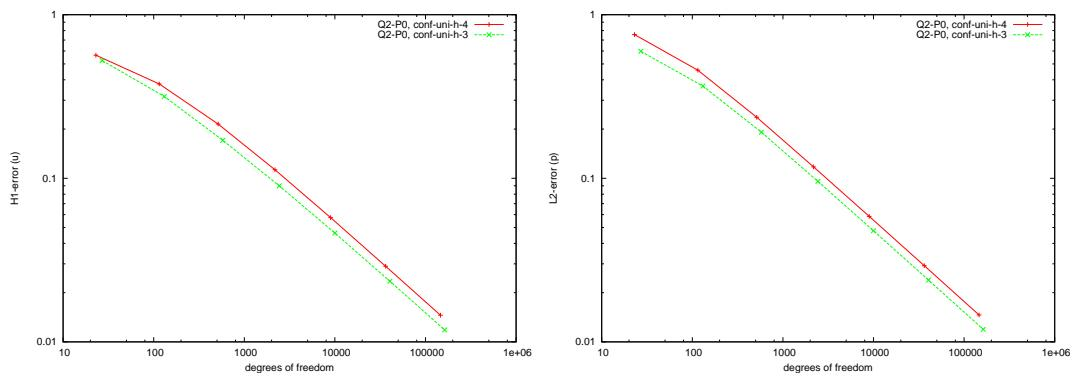
Figure 5.82: Stokes (2d-FEM):  $\|u - u_n\|_{H^1(\Omega)}$  (left) and  $\|p - p_n\|_{L^2(\Omega)}$  (right).
