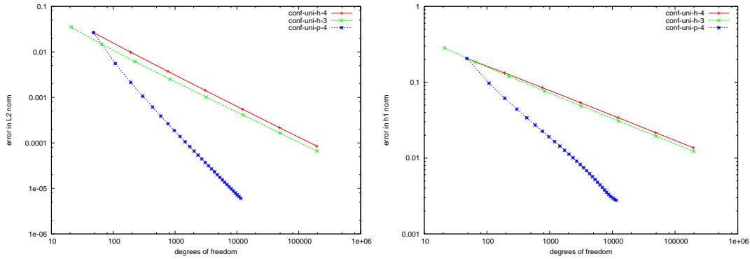
Figure 5.65: Laplace-2d DG:  $\|u - u_n\|_{L^2(\Omega)}$  (left) and  $\|u - u_n\|_{H^1(\Omega)}$  (right).
