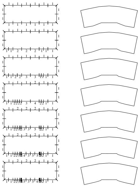
Figure 3.42: hp-adaptive generated meshes for Lamé-BEM (bubble-indicator)
