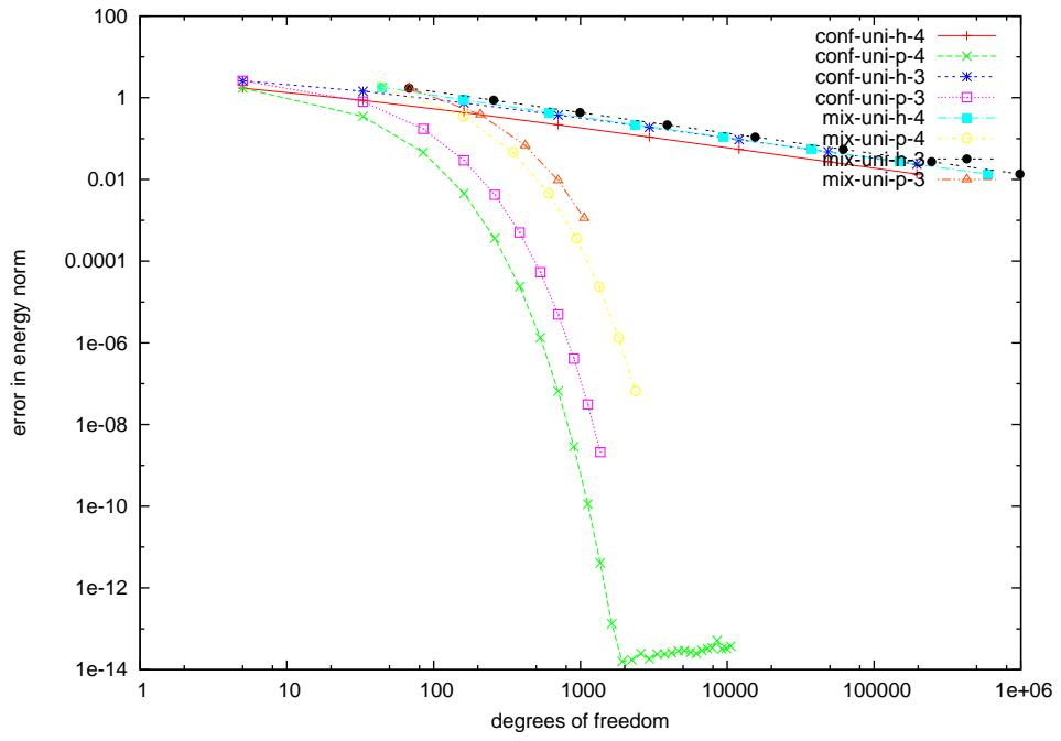
Figure 5.53: Homogenous Dirichlet problem,  $f(x, y) = 2\pi^2 \sin(\pi x) \sin(\pi y)$ .
