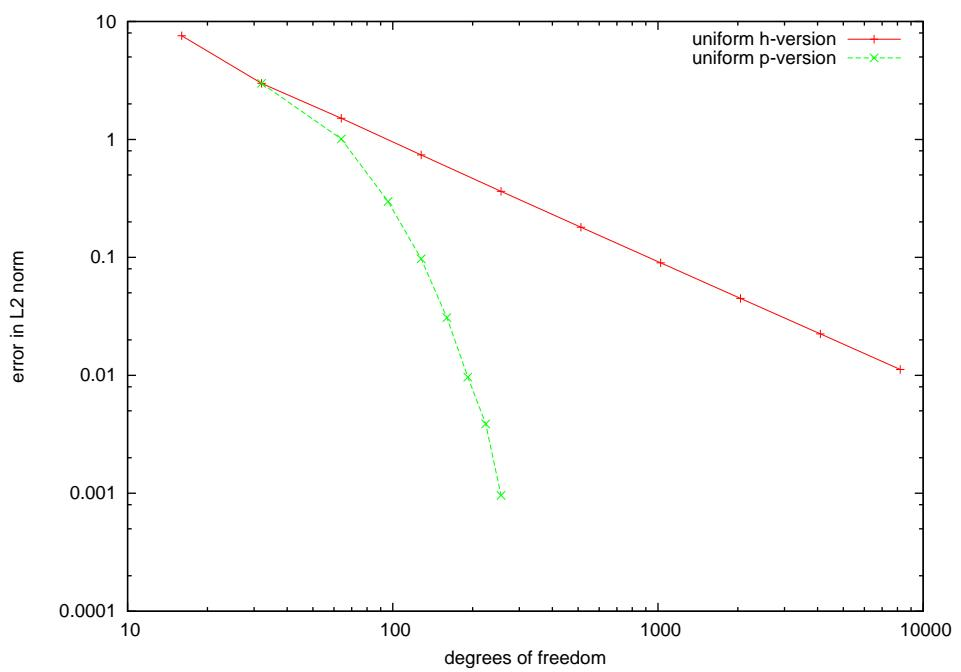
Figure 2.20: Stokes(Dirichlet, exterior): First kind integral equation, convergence in  $L_2$ -norm
