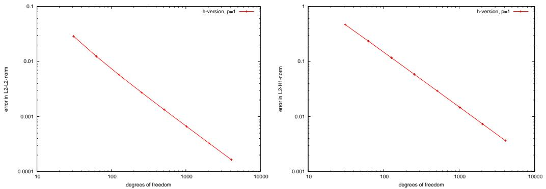
Figure 4.51:  $\|u - u_n\|_{L^2([0,T], L^2(\Omega))}$  (left) and  $\|u - u_n\|_{L^2([0,T], H^1(\Omega))}$  (right) — Heat equation.
