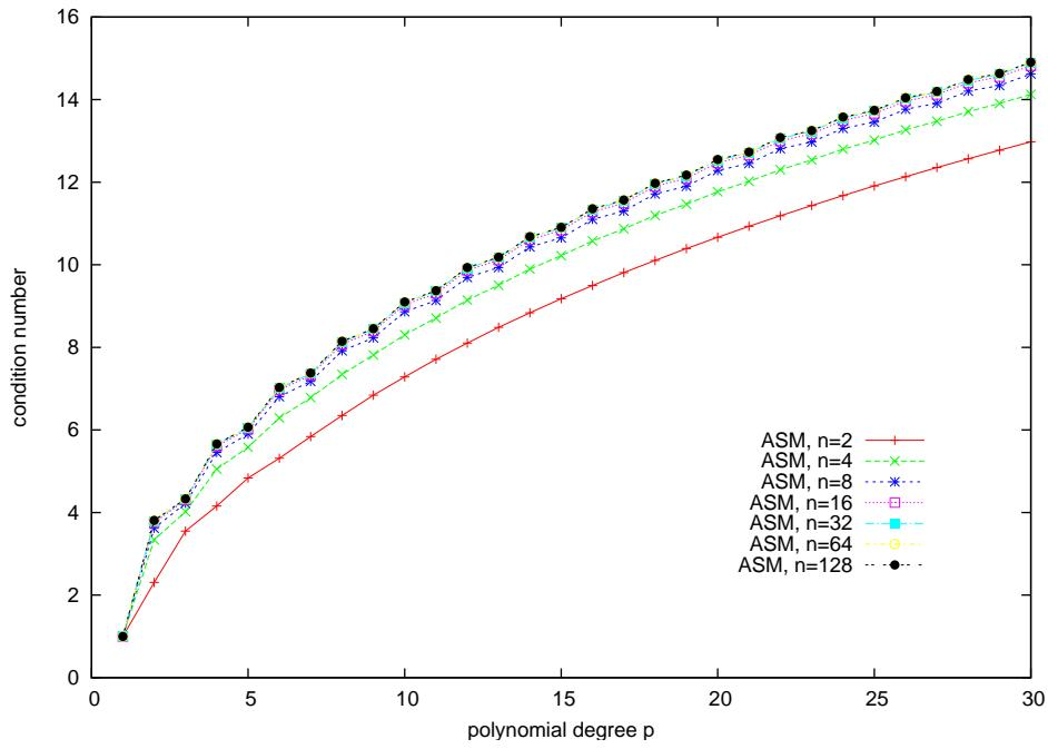
Figure 2.29: Hyper singular integral equation, p-version, condition number
