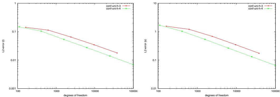
Figure 5.86: Stokes (2d-FEM):  $\|t - t_n\|_{L^2(\Omega)}$  (left) and  $\|\sigma - \sigma_n\|_{L^2(\Omega)}$  (right).
