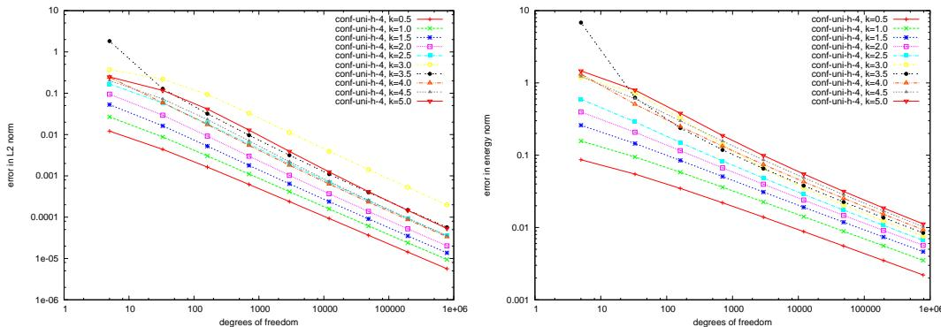
Figure 5.80: Helmholtz (2d-FEM):  $\|u - u_n\|_{L^2(\Omega)}$  (left) and  $\|u - u_n\|_{H^1(\Omega)}$  (right).
