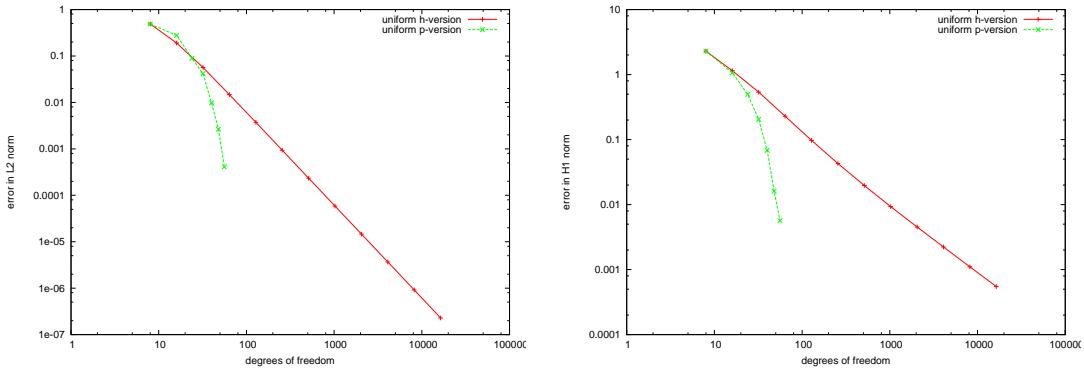
Figure 2.5: Laplace(Neumann): First kind integral equation, convergence in  $L_2$ -norm and  $H^1$ -norm
