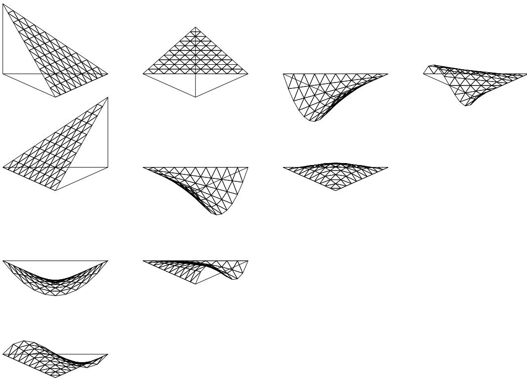
Figure 1.164: Base functions on triangles (continuous)
