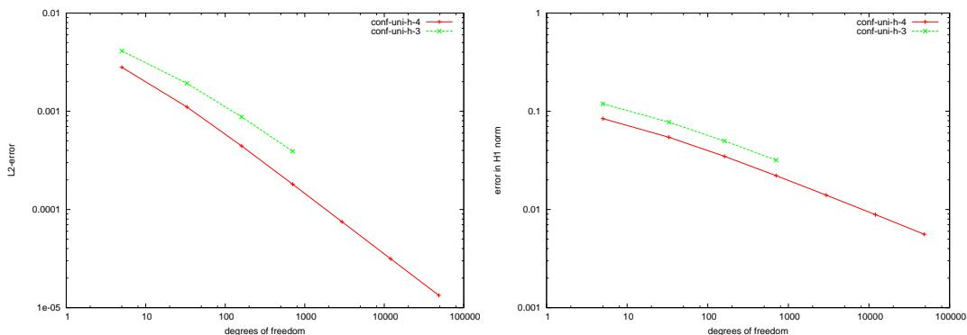
Figure 5.64:  $\|u - u_n\|_{L^2(\Omega)}$  (left) and  $\|u - u_n\|_{H^1(\Omega)}$  (right) — p-Laplacian.
