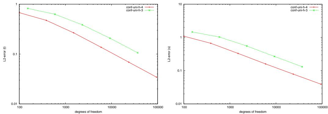
Figure 5.84: Stokes (2d-FEM):  $\|t - t_n\|_{L^2(\Omega)}$  (left) and  $\|\sigma - \sigma_n\|_{L^2(\Omega)}$  (right).
