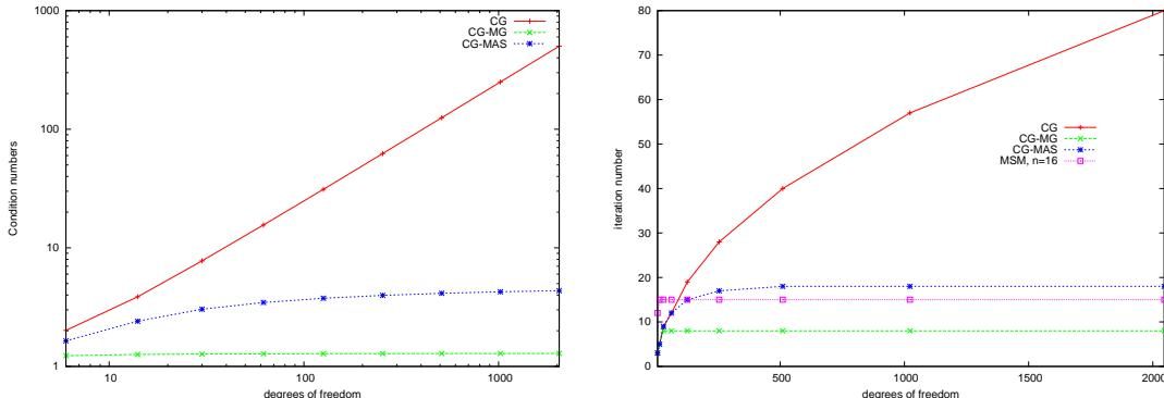
Figure 2.35: Hypersingular Lamé integral equation, condition number and iteration numbers of multilevel preconditioners
