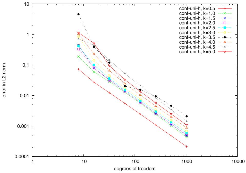
Figure 2.17: Helmholtz: Second kind integral equation, convergence in  $L_2$ -norm
