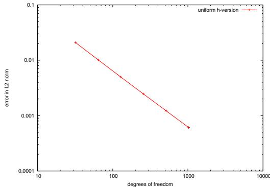
Figure 2.12: Lame(Dirichlet, interior, traction): Steklov-Operator, convergence in  $L_2$ -norm
