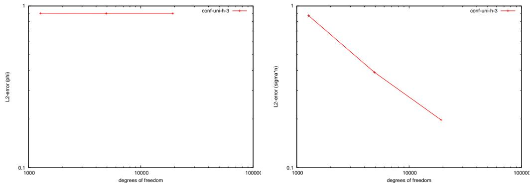
Figure 6.121: Stokes (2d-FEM-BEM):  $\|\phi - \phi_n\|_{L^2(\Gamma)}$  (left) and  $\|\sigma \cdot \vec{n} - \sigma_n \cdot \vec{n}\|_{L^2(\Gamma)}$  (right).
