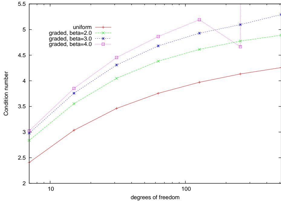
Figure 2.36: Hypersingular integral equation, algebraically graded  $h$  version with Multilevel Schwarz preconditioner, condition number  $\kappa(P_{\text{ASM}})$
