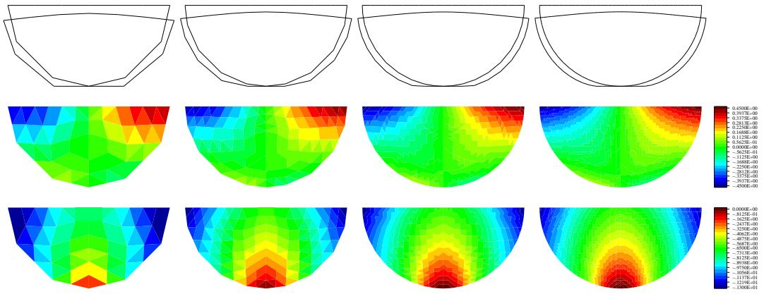
Figure 3.44: Deformed body (top), deformation in x (middle), deformation in y (bottom)
