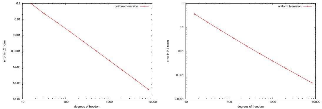
Figure 2.9: Lame(Neumann, exterior): First kind integral equation, convergence in  $L_2$ -norm and  $H^1$ -norm
