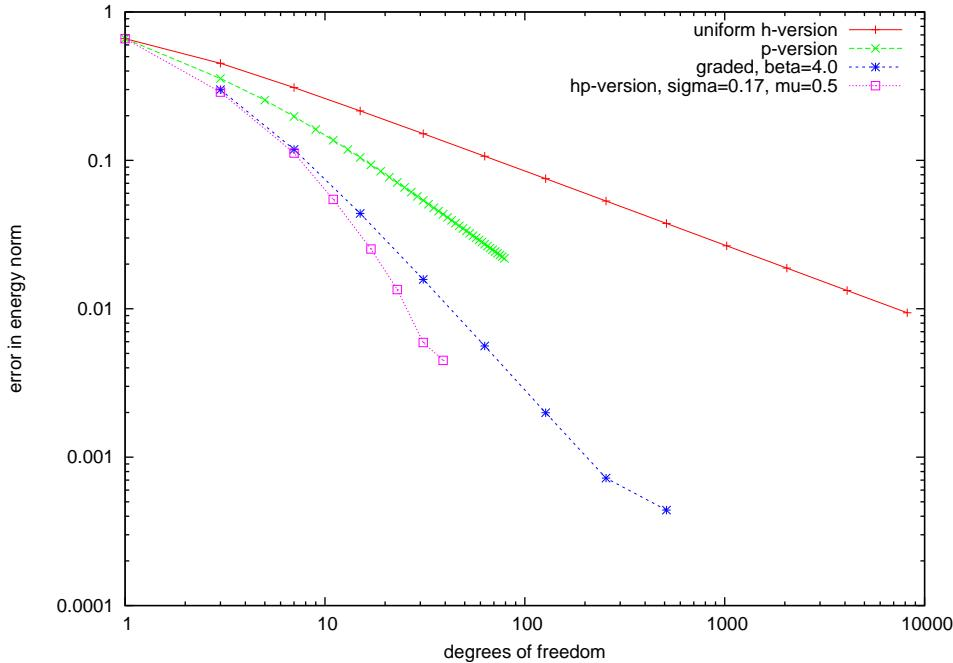
Figure 2.4: Hyper-singular integral equation, convergence in energy norm
