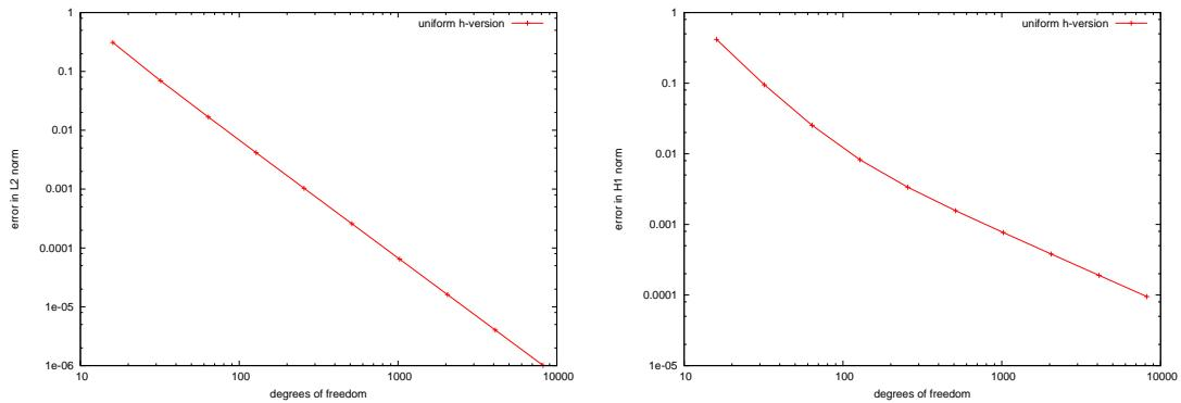
Figure 2.21: Stokes(Neumann): First kind integral equation, convergence in  $L_2$ -norm and  $H^1$ -norm
