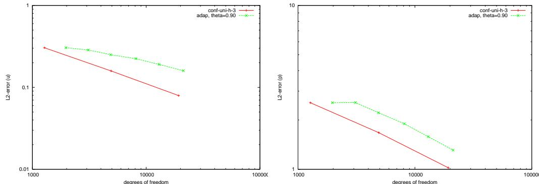
Figure 6.122: Stokes (2d-FEM-BEM):  $\|u - u_n\|_{L^2(\Omega)}$  (left) and  $\|p - p_n\|_{L^2(\Omega)}$  (right).
