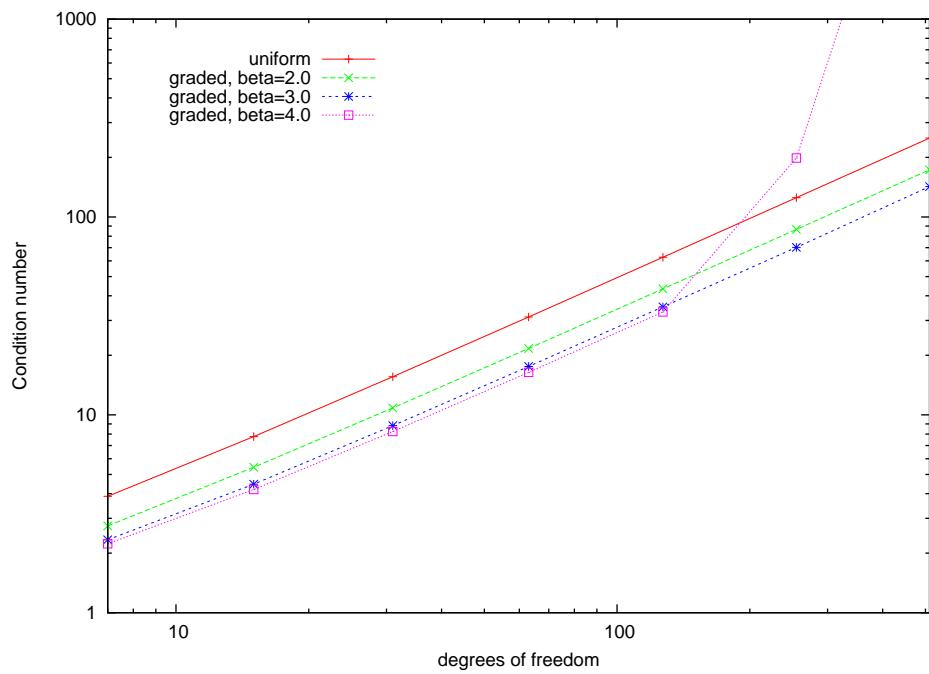
Figure 2.37: Hypersingular integral equation, algebraically graded  $h$  version without preconditioner, condition number  $\kappa(A_N)$
