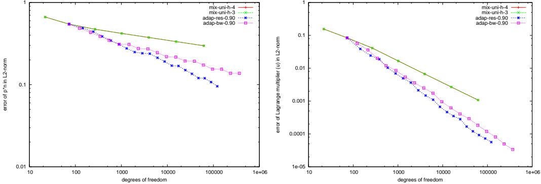
Figure 5.60:  $\|p \cdot \vec{n} - p_n \cdot \vec{n}\|_{L^2(\Gamma)}$  (left) and  $\|(-u) - \lambda_n\|_{L^2(\Gamma_N)}$  (right) — Mixed Neumann problem.
