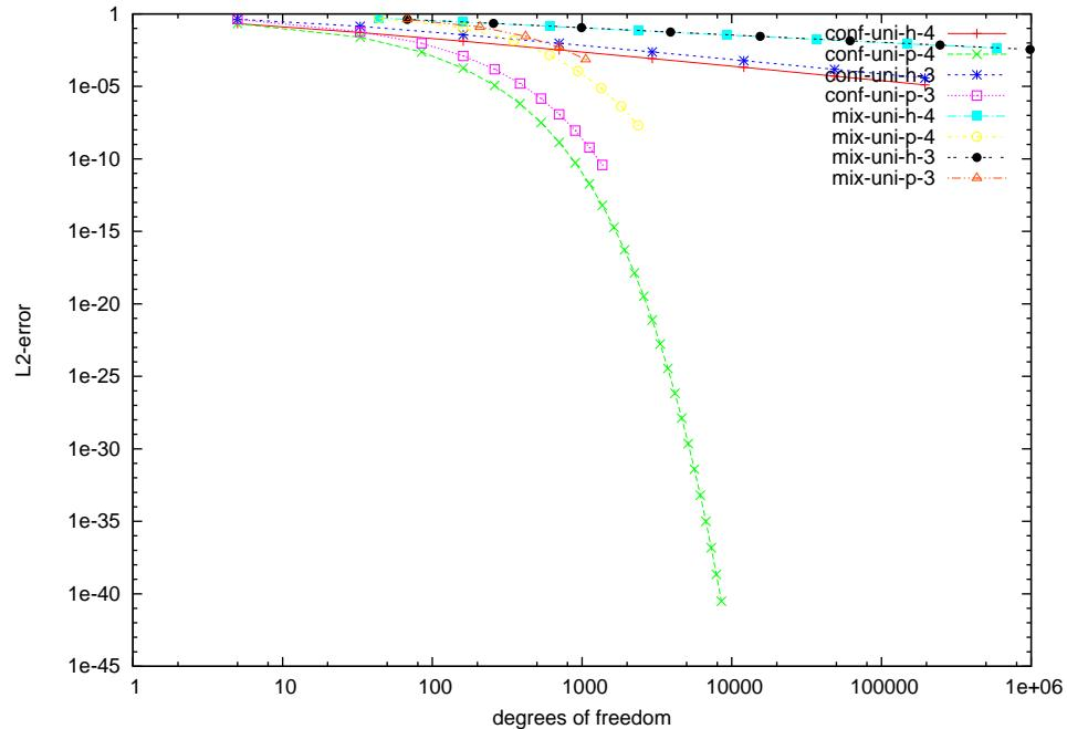
Figure 5.69: Homogenous Dirichlet problem,  $f(x, y) = 2\pi^2 \sin(\pi x) \sin(\pi y)$ .
