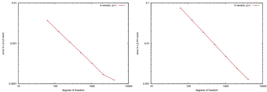
Figure 4.52:  $\|u - u_1^n\|_{L^2([0,T],L^2(\Omega))}$  (left) and  $\|u - u_1^n\|_{L^2([0,T],H^1(\Omega))}$  (right) — Wave equation.
