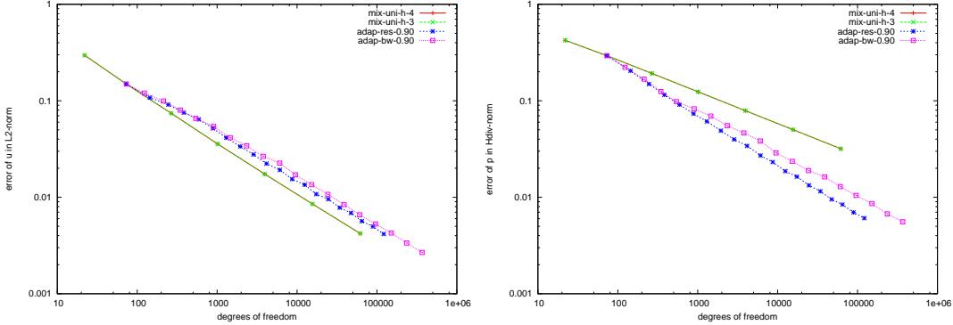
Figure 5.59:  $\|u - u_n\|_{L^2(\Omega)}$  (left) and  $\|p - p_n\|_{H(\text{div};\Omega)}$  (right) — Mixed Neumann problem.
