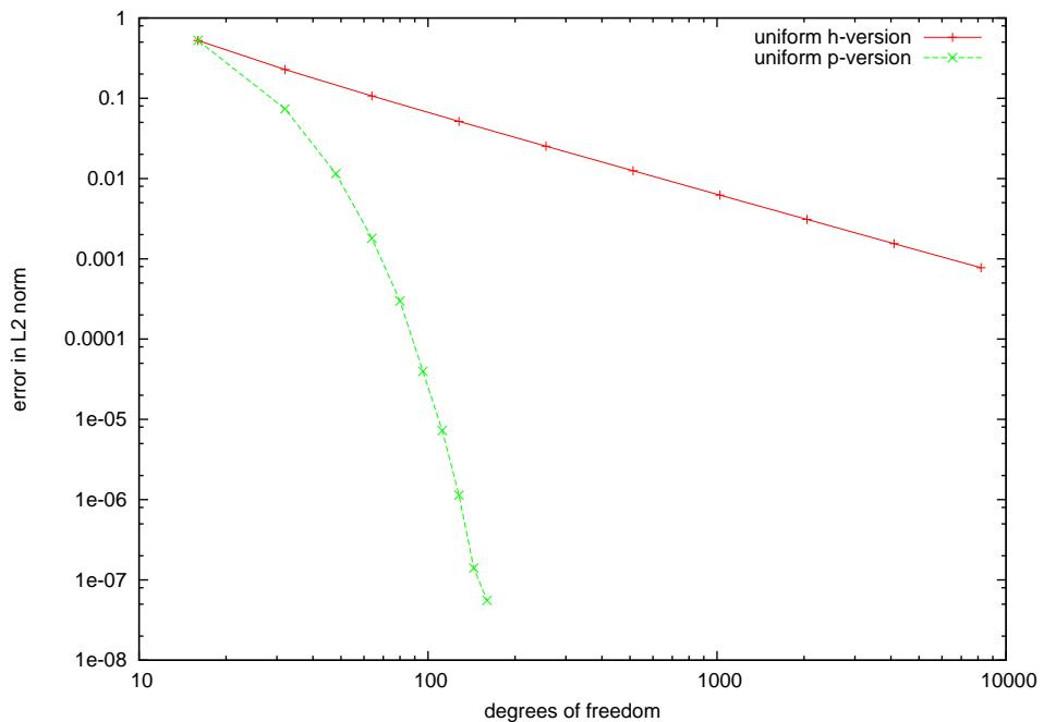
Figure 2.19: Stokes(Dirichlet): First kind integral equation, convergence in  $L_2$ -norm
