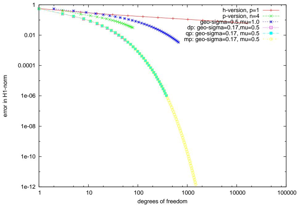
Figure 4.46: Homogenous Dirichlet problem,  $\alpha = 0.7$ .
