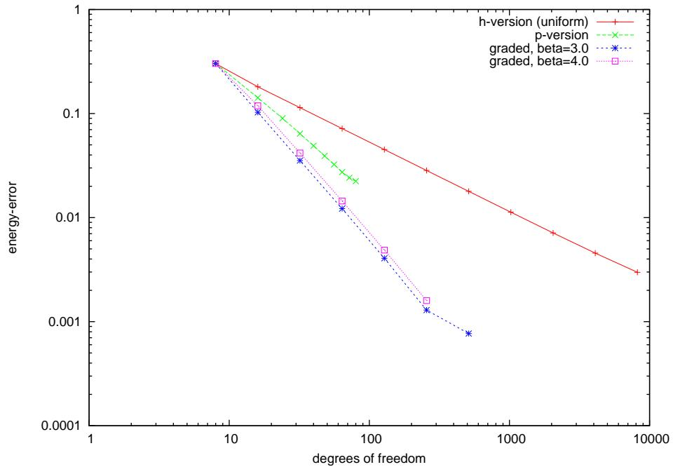
Figure 2.3: Weakly singular integral equation, convergence in energy-norm
