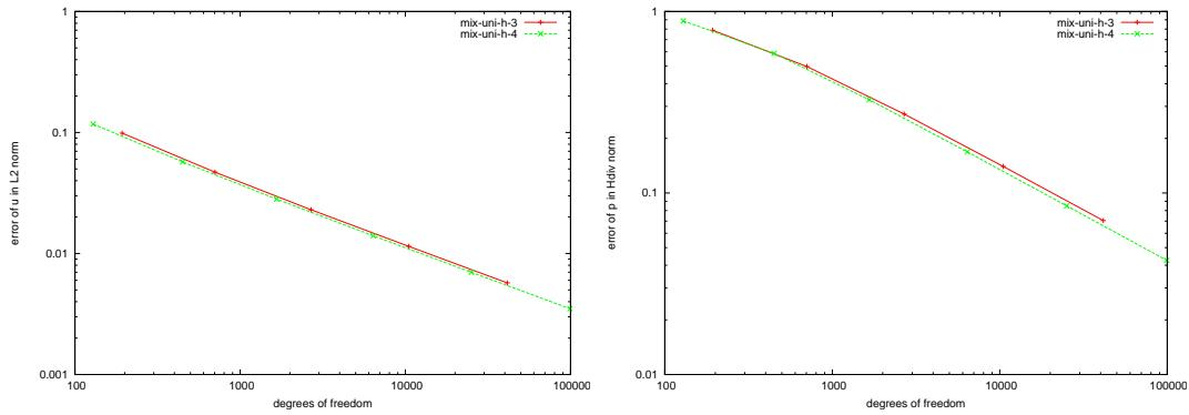
Figure 6.111: Error of  $u$  in L2-norm (left) and Error of  $p$  in Hdiv-norm (right)
