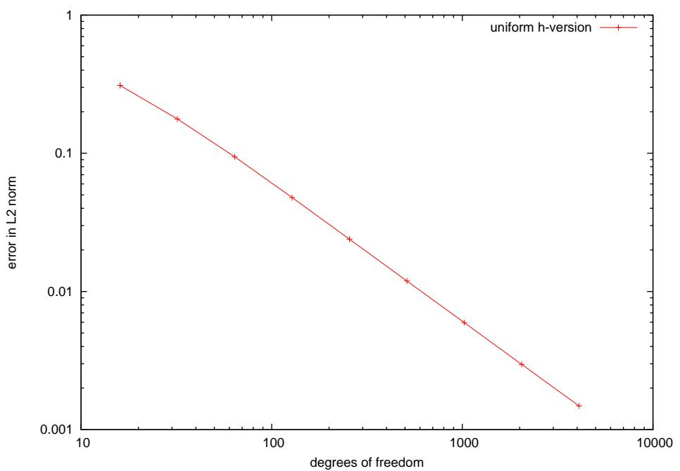
Figure 2.8: Lame(Dirichlet, exterior): First kind integral equation, convergence in  $L_2$ -norm
