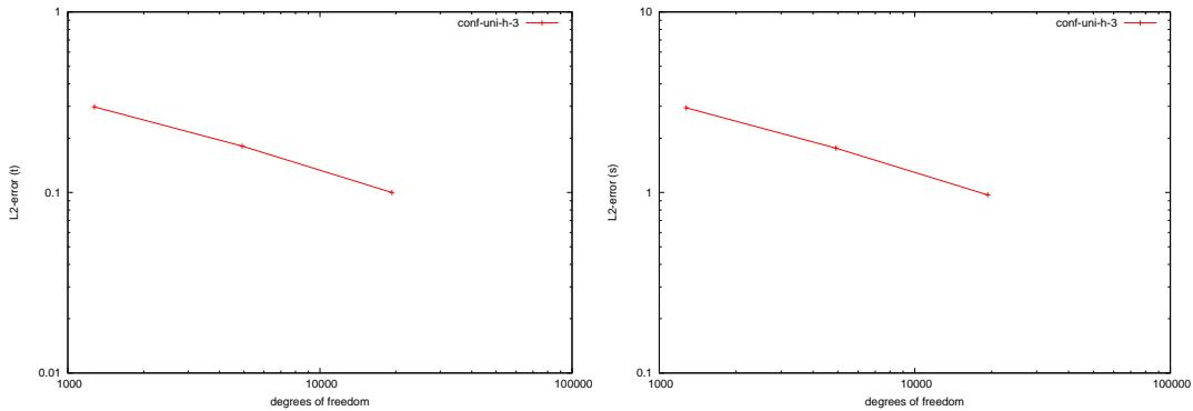
Figure 6.120: Stokes (2d-FEM-BEM):  $\|t - t_n\|_{L^2(\Omega)}$  (left) and  $\|\sigma - \sigma_n\|_{L^2(\Omega)}$  (right).
