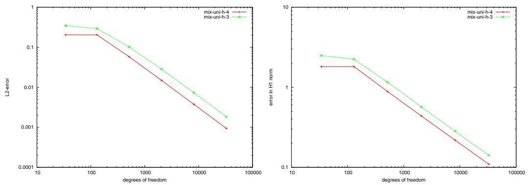
Figure 5.81:  $\|u - u_n\|_{L^2(\Omega)}$  (left) and  $\|u - u_n\|_{H^1(\Omega)}$  (right) — Clamped plate.
