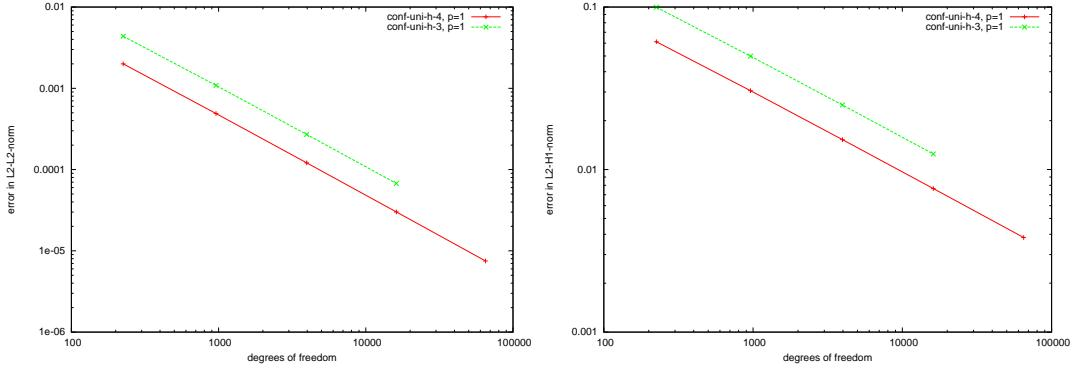
Figure 5.101:  $\|u - u_n\|_{L^2([0,T], L^2(\Omega))}$  (left) and  $\|u - u_n\|_{L^2([0,T], H^1(\Omega))}$  (right) — Heat equation.
