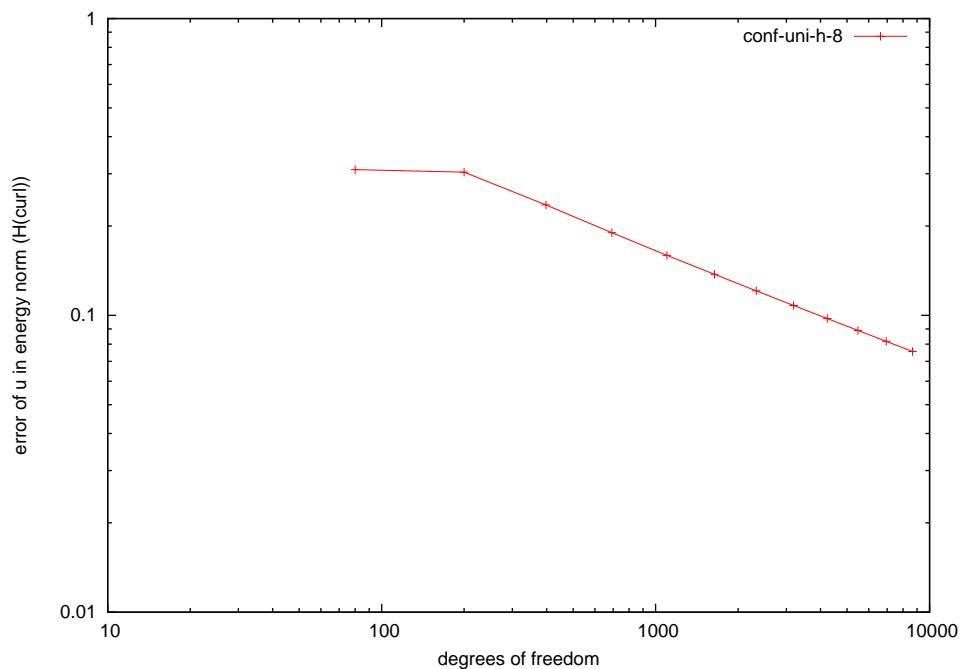
Figure 10.162: Error of  $u$  in  $H(\text{curl}, \Omega)$ -norm.
