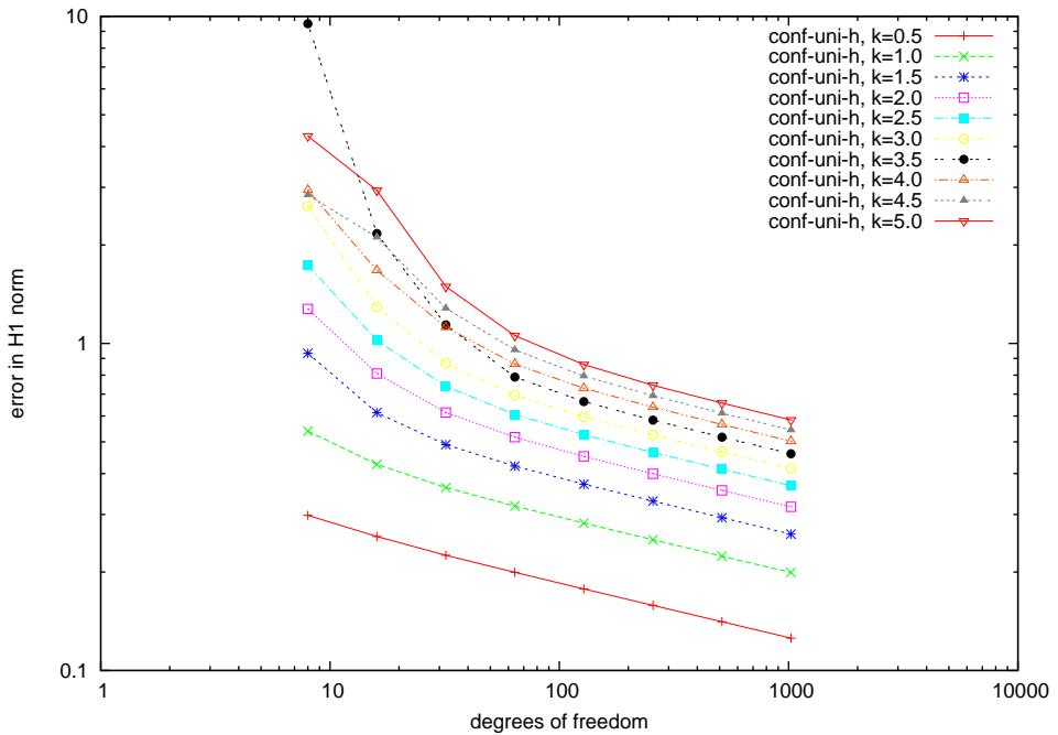
Figure 2.16: Helmholtz: Hypersingular integral equation, convergence in  $H^1$ -norm
