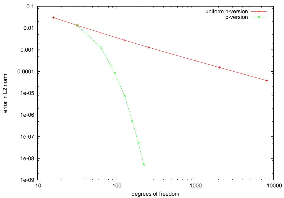
Figure 2.6: Lame(Dirichlet, interior): First kind integral equation, convergence in  $L_2$ -norm
