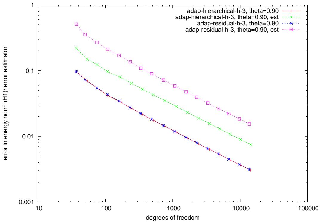
Figure 6.106: FEM-BEM Coupling on the L-Shape, Error estimators
