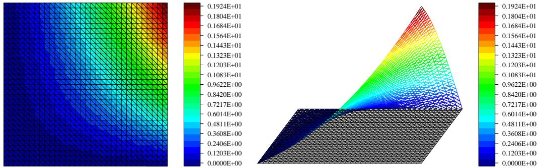
Figure 5.93: Plot of the Galerkin solution  $u(x, y) = \exp(x) \sin(x) \sin(y)$
