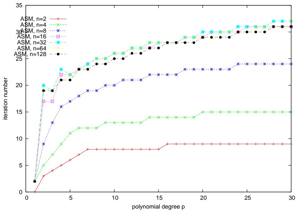
Figure 2.30: Hyper singular integral equation, p-version, iteration numbers
