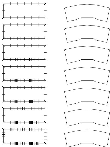
Figure 3.41:  $h$ -adaptive generated meshes for Lamé-BEM (bubble-indicator)
