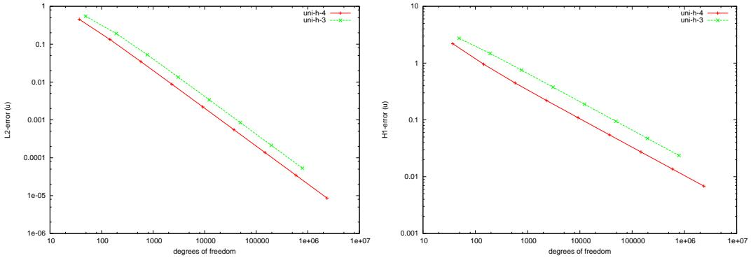
Figure 5.70: Laplace (L2-Least Squares):  $\|u - u_n\|_{L^2(\Omega)}$  (left) and  $|u - u_n|_{H^1(\Omega)}$  (right).
