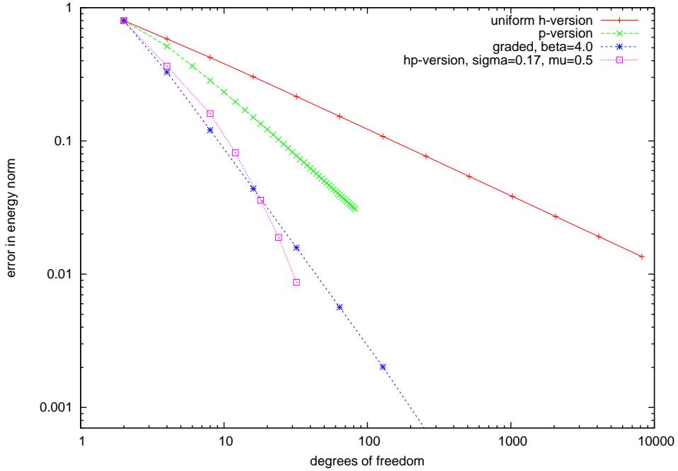
Figure 2.1: Weakly singular integral equation, convergence in energy norm
