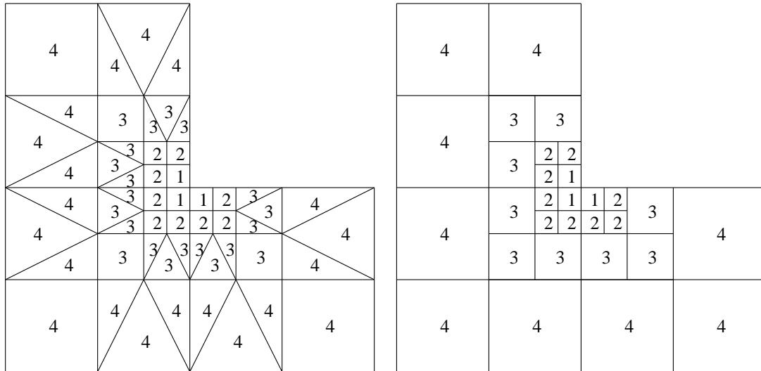
Figure 5.56: Conforming geometric mesh (left) and geometric mesh with hanging nodes (right)
