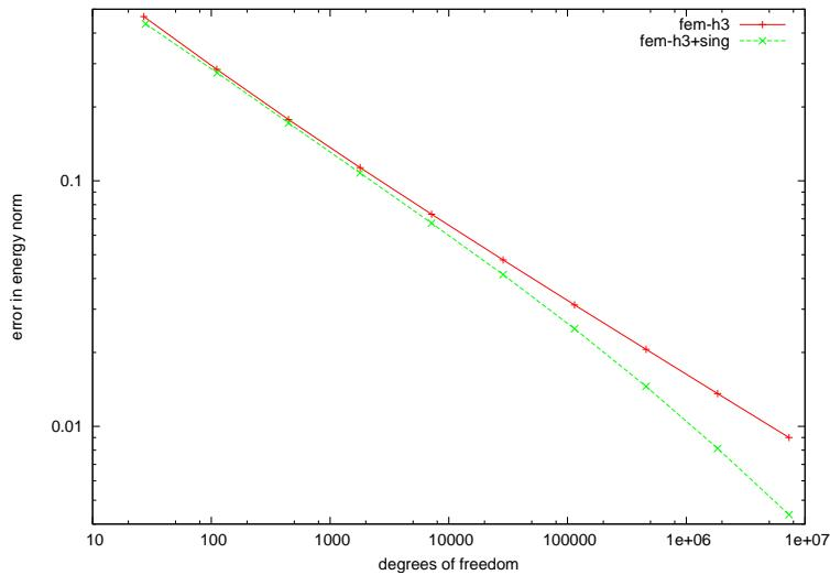
Figure 5.62: Energy error for fem without/with singularity function at tip.
