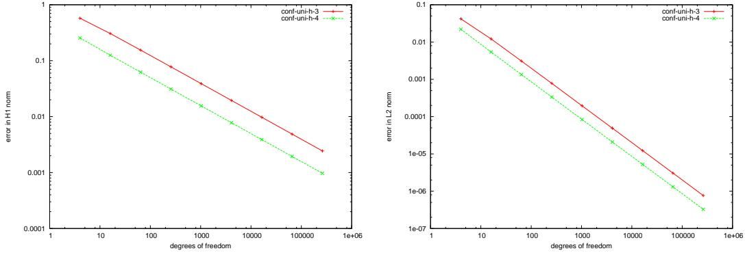
Figure 5.92: Error in  $H^1(\Omega)$ -norm (left) and in  $L^2(\Omega)$ -norm (right)
