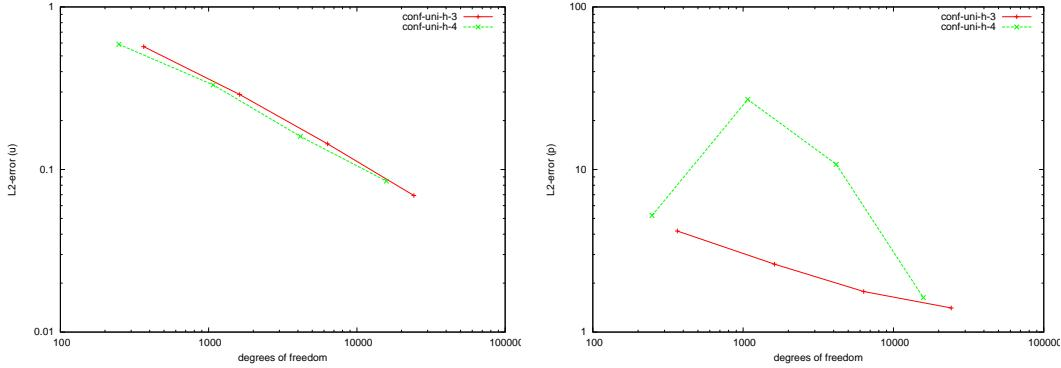
Figure 5.87: Stokes (2d-FEM):  $\|u - u_n\|_{L^2(\Omega)}$  (left) and  $\|p - p_n\|_{L^2(\Omega)}$  (right).
