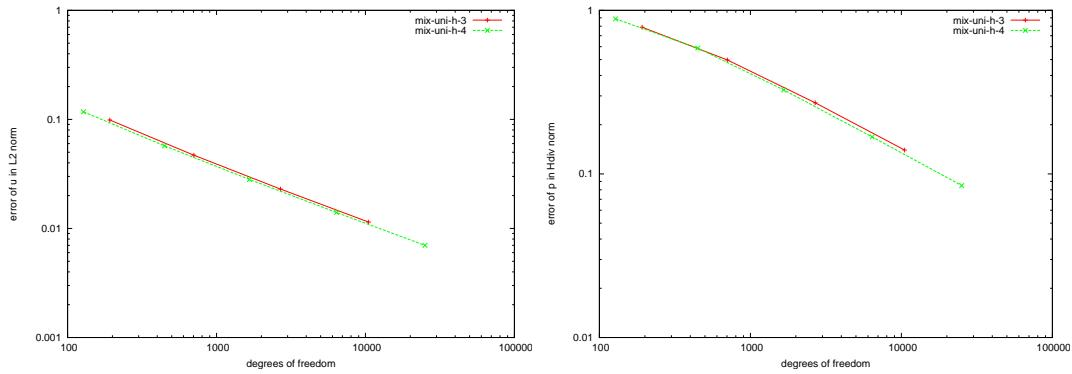
Figure 6.109: Error of  $u$  in L2-norm (left) and Error of  $p$  in Hdiv-norm (right)
