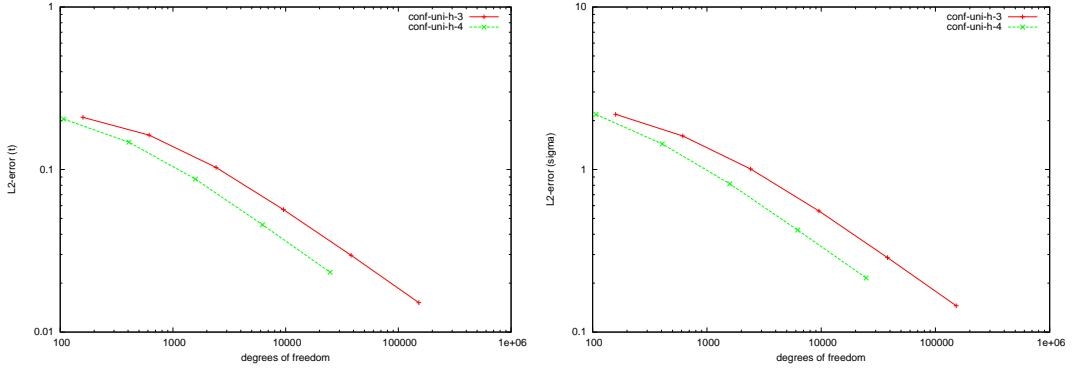
Figure 5.90: Stokes (2d-FEM, mixed b.c.):  $\|t - t_n\|_{L^2(\Omega)}$  (left) and  $\|\sigma - \sigma_n\|_{L^2(\Omega)}$  (right).
