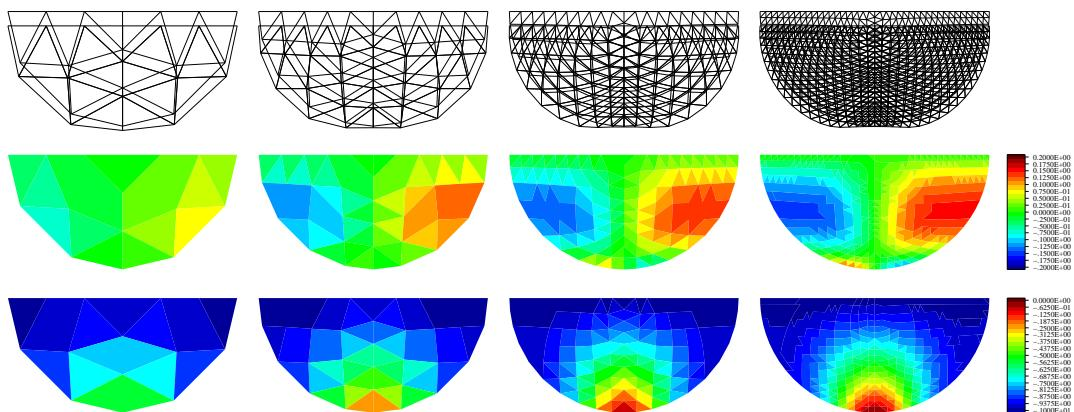
Figure 3.45: Deformed body (top), deformation in x (middle), deformation in y (bottom)
