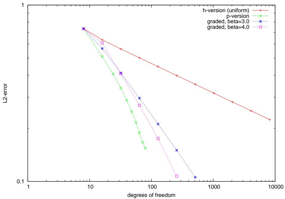
Figure 2.2: Weakly singular integral equation, convergence in  $L_2$ -norm
