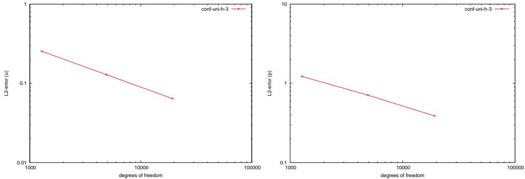
Figure 6.119: Stokes (2d-FEM-BEM):  $\|u - u_n\|_{L^2(\Omega)}$  (left) and  $\|p - p_n\|_{L^2(\Omega)}$  (right).
