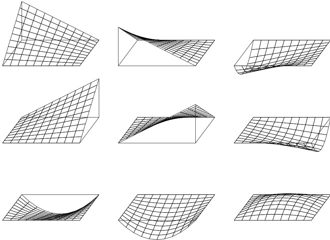
Figure 1.163: Base functions on quadrilaterals (continuous)
