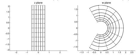
The circles and radial lines are curves where the real and imaginary parts of Log(w) are constant. These are orthogonal.
