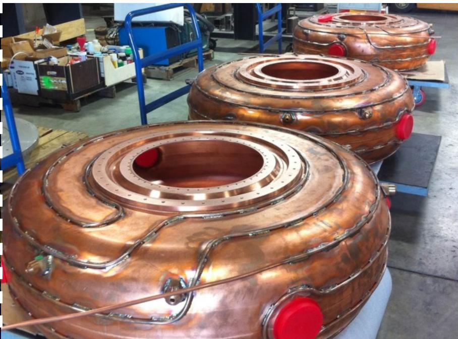
MICE Normal Conducting RF Cavities
