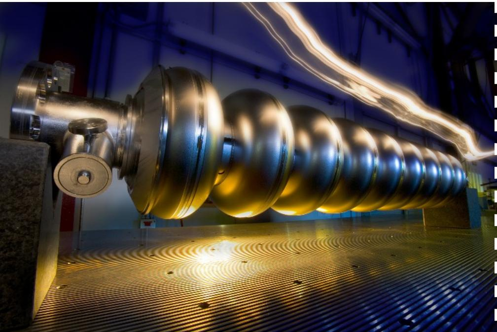
ILC Superconducting RF Cavities
