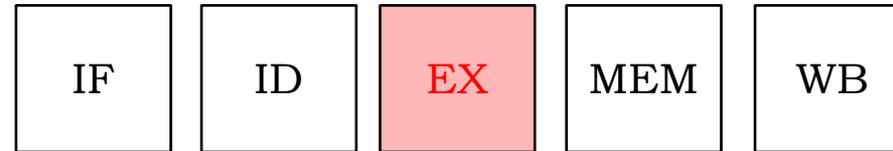
Here the ALU operates on the operands which have been prepared in the decode cycle
