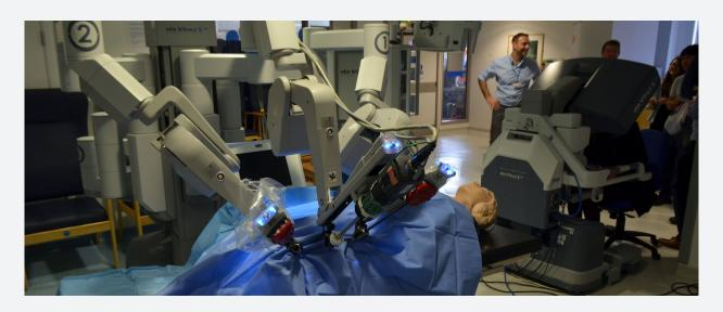
▲ Figure 4: A da Vinci Robot Surgical System on display at Addenbrooke's Treatment Centre, Cambridge, during the 2015 Cambridge Science Festival. Although autonomous surgical robots are not currently in use, robots are already assisting surgical procedures, and the data being gathered from the use of this technology can be used to train surgeons or to improve surgical techniques. (Image used under the Creative Commons Attribution-Share Alike 3.0 Unported license)
