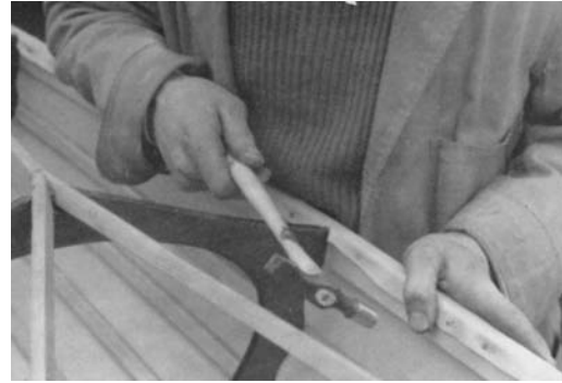
8. Tacking the hull fabric to the gunwale – note the supporting hand.
