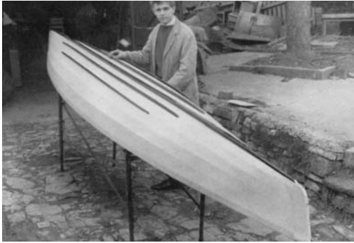
7. The hull covered; keel and bilge keels fitted
